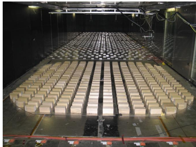
Figure 1. A 21x14 array of 14x7x7cm blocks installed on the turntable in the EnFlo wind tunnel.
